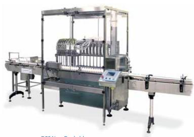
**DFS Non-Dockable Filling Machine** Flexible Design, Wide Range of Filamatic Piston Pump Sizes, Product Viscosities, and Speeds
